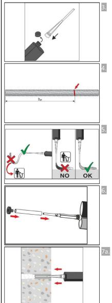
Screw on static-mixing nozzle and load the cartridge into an appropriate dispensing tool.
