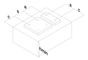
Fixing points with a spacing a  $\leq$  s<sub>cr,N</sub> are considered as a group with a maximum characteristic resistance N<sub>Rk,p</sub> acc. to Table 17 – Table 27. For a spacing a > s<sub>cr,N</sub> the anchors are considered as single anchors, each with a characteristic resistance N<sub>Rk,p</sub> acc. to Table 17 – Table 27.
