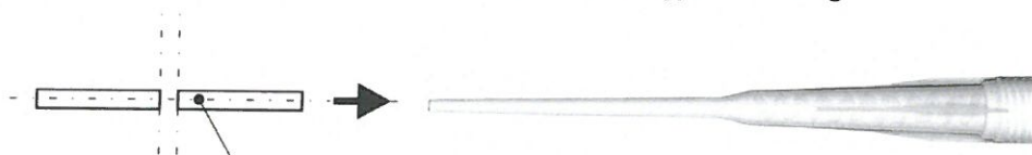
additional mixer extension, variable length between 300 mm up to 1000 mm
